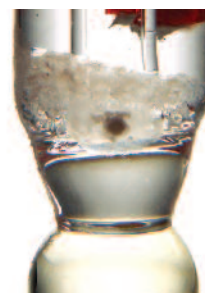
KCl Crystals Blocking Reference Junction
