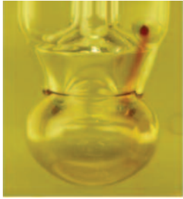
Correctly Functioning Ceramic Junction Outflow of Electrolyte (Red Dye)
